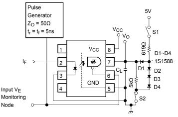
$\ensuremath{\mathsf{C}}_{\ensuremath{\mathsf{L}}}$  is approximately 15pF which includes probe and stray wiring capacitance.
