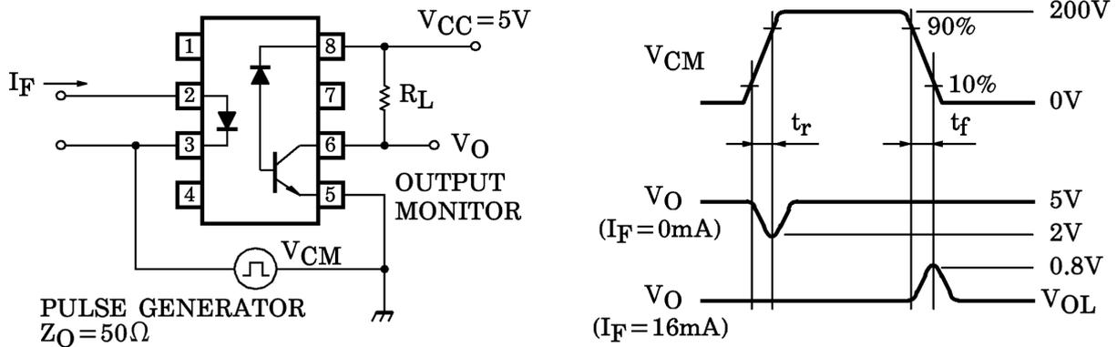
$$CM_H = \frac{160 (V)}{t_r (\mu s)}, \quad CM_L = \frac{160 (V)}{t_f (\mu s)}$$
