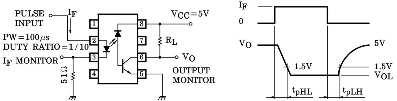
**Test Circuit 2: Common Mode Noise Immunity Test Circuit**
