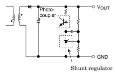
This circuit amplifies the difference between the switching power supply's secondary output voltage and the shunt regulator's reference voltage. It then feeds the amplified voltage back to the primary input voltage via the photocoupler.
