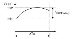
$$\left| \alpha V_{REF} \right| = \frac{\left( \frac{V_{REF (dev)} \times 10^6}{V_{REF} @25^{\circ}C} \right)}{\Delta Ta} (ppm/^{\circ}C)$$
