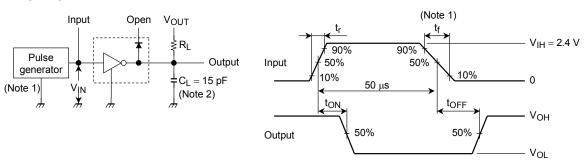
Note 1: Pulse Width 50  $\mu$ s, Duty Cycle 10% Output Impedance 50  $\Omega,\,t_{\Gamma}\leq$  5 ns,  $t_{f}\leq$  10 ns
