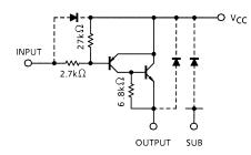
Note: The input and output parasitic diodes cannot be used as clamp diodes.
