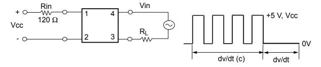
(Note 3): In-pulse noise durability test circuit
