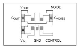
Circuit board material: glass epoxy, Circuit board dimension: 30 mm  $\times$  30 mm, Copper foil pad area: 50 mm<sup>2</sup> (t = 0.8 mm)
