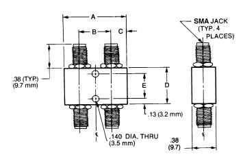
All dimensions are ± .020 except mounting diameters (± .005) and mounting hole location (± .010).
