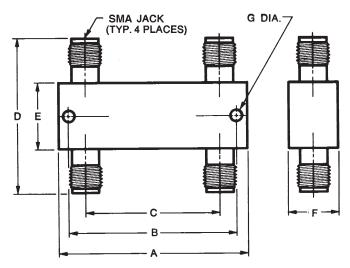
All dimensions are ± .020 except mounting diameters (± .005) and mounting hole location (± .010).
