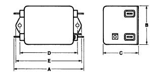
Typical dimensions Terminals:  $\frac{.250}{6.35}$ (5) Holes:  $\frac{.07}{7.8}$  Dia.(4) Slot:  $\frac{.07 \times .16}{7.8 \times 4.1}$ Mounting holes:  $\frac{.188}{4.78}$  Dia. (2)
