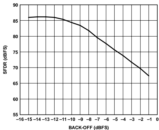
Figure 10. SFDR vs. Backoff @ AIN with f_{IN} = 70 MHz
