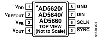
Figure 4. MSOP Pin Configuration
