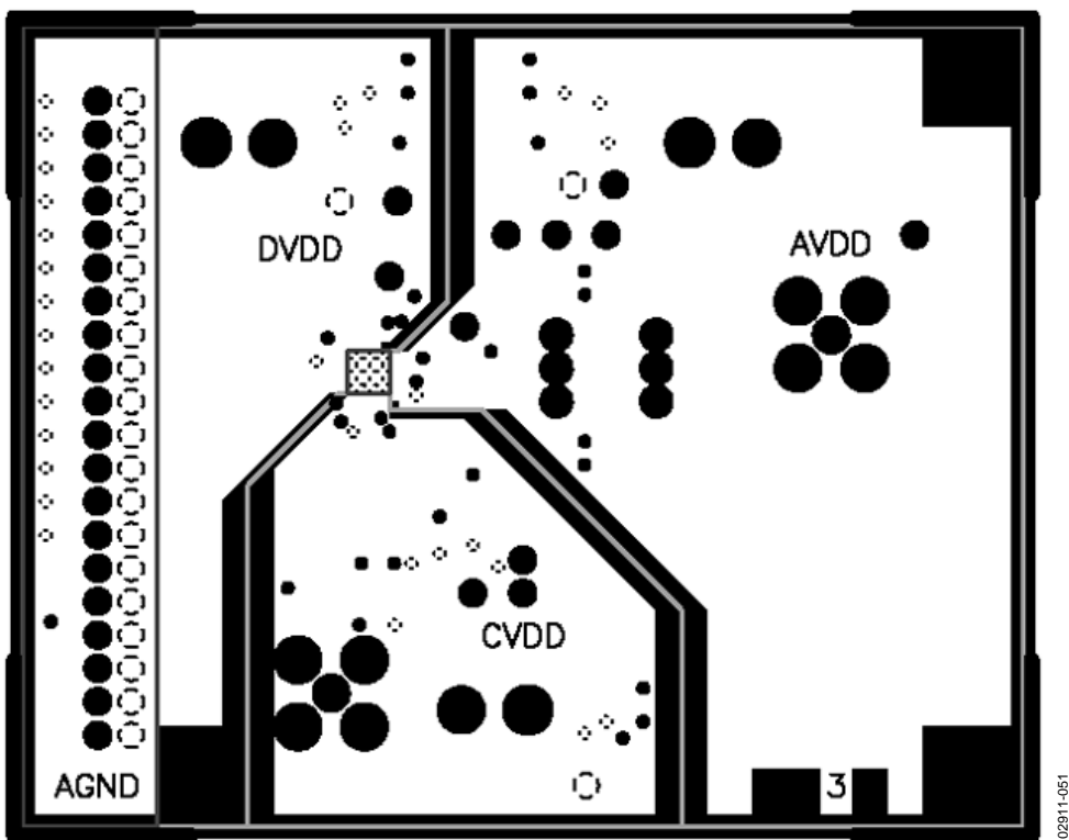
Figure 53. LFCSP Evaluation Board Layout—Power Plane
