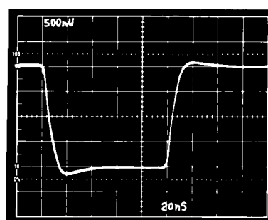
Figure 14. Small Signal Pulse Response, Gain = -1 , R_1 = R_2 = 1 \text{ k}\Omega
