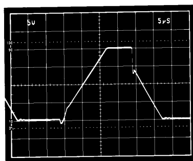
Figure 19b. Unity Gain Follower Pulse Response (Large Signal)
