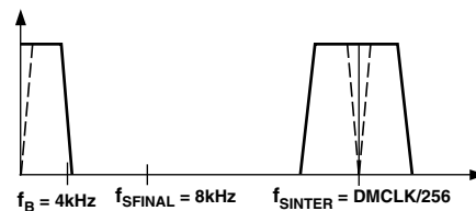
d. Final Filter LPF (HPF) Transfer Function
