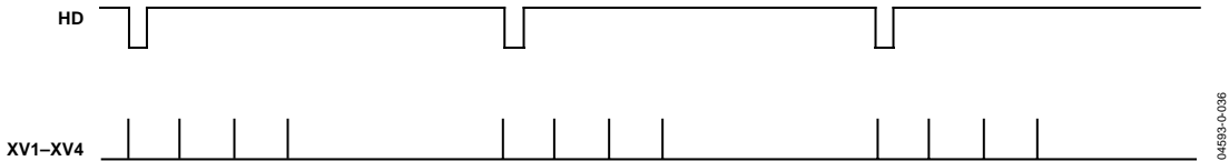
Figure 35. Nonoverlapping Example while Operating in Normal Vertical Timing Operation SVREP_MODE = 0 and VTPREPx = 4
