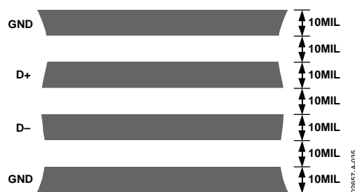
Figure 35. Arrangement of Signal Tracks
