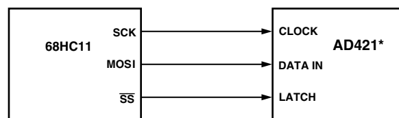
Figure 8. AD421 to 68HC11 Interface
