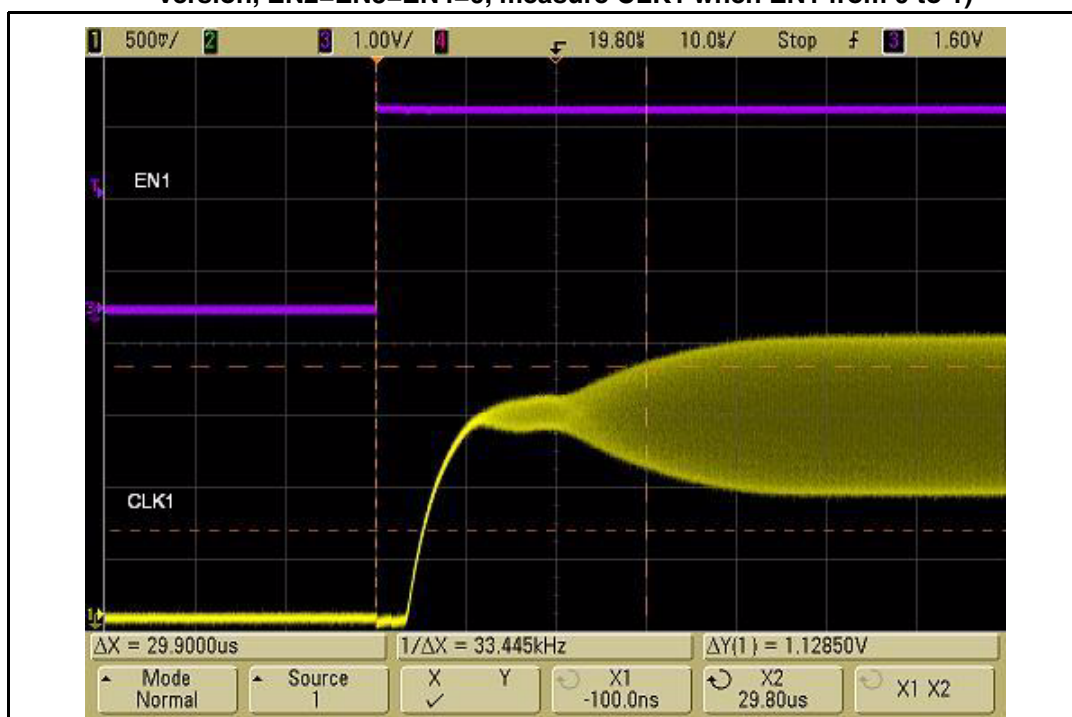
Figure 17. STCD10x0 recovery time from standby to active (STCD1040, 2.8 V version, EN2=EN3=EN4=0, measure CLK1 when EN1 from 0 to 1)
