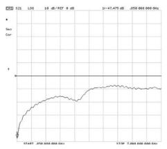
Insertion loss tested to 7 GHz for the CRFReed Relay but with the internal Reed Switch replaced with a bare copper wire. Horizontal full scale: 7.0 GHz. Vertical scale: 10 dB/div referenced from the 0 mark. Isolation tested to 7 GHz for the CRF Reed Relay. Horizontal full scale: 7.0 GHz. Vertical scale: 10 dB/div referenced from the 0 mark.
