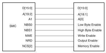
Figure 21-5. Memory Connection for a 32-bit Data Bus
