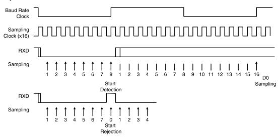
Figure 33-9. Asynchronous Character Reception
