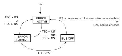
An error active unit takes part in bus communication and sends an active error frame when the CAN controller detects an error.
