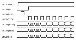
Figure 43-7. Single Scan Monochrome and Color 4-bit Panel Timing (First Line Expanded View)
