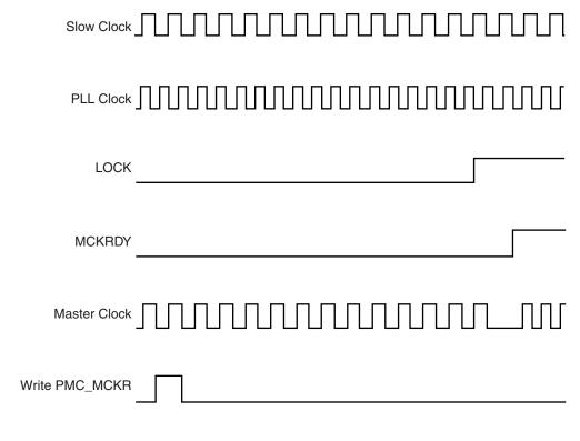
Figure 27-4. Switch Master Clock from Main Clock to Slow Clock
