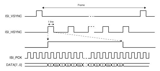
Figure 45-4. SAV and EAV Sequence Synchronization
