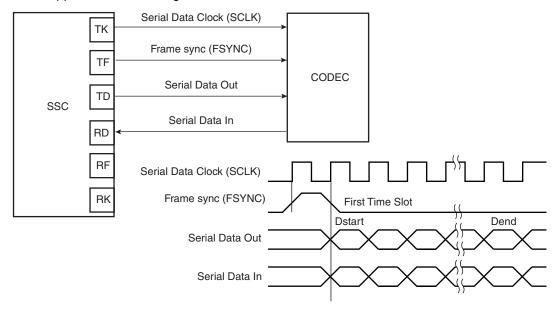
Figure 34-19. Time Slot Application Block Diagram
