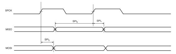
Figure 46-8. SPI Master Mode with (CPOL=0 and NCPHA=1) or (CPOL=1 and NCPHA=0)
