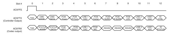
Table 35-2. AC-link Output Slots Transmitted from the AC'97C Controller
