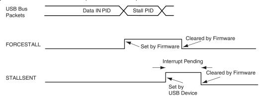
Figure 42-14. Stall Handshake (Data OUT Transfer)
