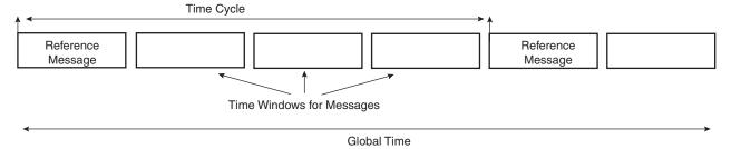
Time Trigger Mode is enabled by setting the TTM field in the CAN\_MR register. In Time Triggered Mode, as in Timestamp Mode, the CAN\_TIMESTP field captures the values of the internal counter, but the MTIMESTAMP fields in the CAN\_MSRx registers are not active and are read at 0.
