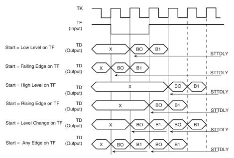
Figure 34-11. Receive Pulse/Edge Start Modes
