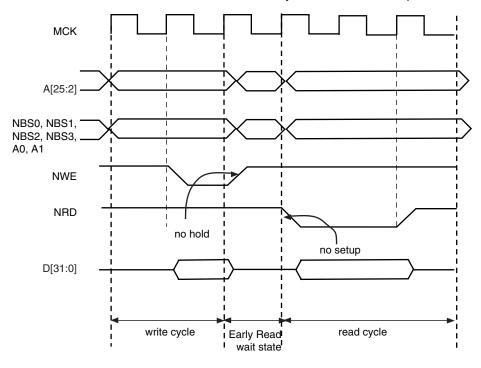
Figure 21-18. Early Read Wait State: NCS Controlled Write with No Hold Followed by a Read with No NCS Setup
