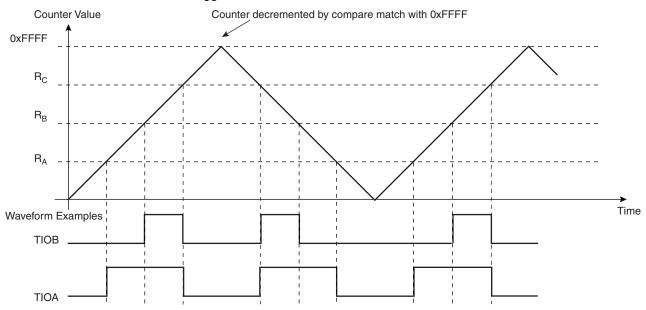
Figure 36-12. WAVSEL = 01 With Trigger
