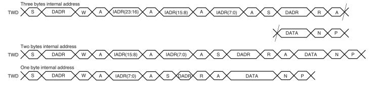
Figure 32-8. Master Read with One Byte Internal Address and Multiple Data Bytes
