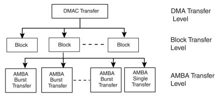
**Block:** A block of DMAC data. The amount of data (block length) is determined by the flow controller. For transfers between the DMAC and memory, a block is broken directly into a sequence of AMBA bursts and AMBA single transfers. For transfers between the DMAC and a non-memory peripheral, a block is broken into a sequence of DMAC transactions (single and bursts). These are in turn broken into a sequence of AMBA transfers.
