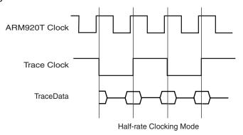
Care must be taken on the choice of the trace capture system as it needs to support half-rate clock functionality.
