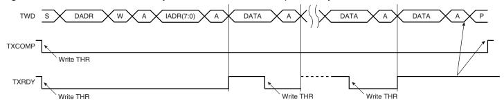
Figure 32-7. Master Read with One, Two or Three Bytes Internal Address and One Data Byte
