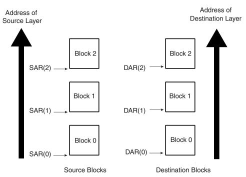
If the user needs to execute a DMA transfer where the source and destination address are contiguous but the amount of data to be transferred is greater than the maximum block size DMAC\_CTLx.BLOCK\_TS, then this can be achieved using the type of multi-block transfer as shown in Figure 24-7 on page 273.
