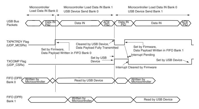
**Warning:** There is software critical path due to the fact that once the second bank is filled, the driver has to wait for TX\_COMP to set TX\_PKTRDY. If the delay between receiving TX\_COMP is set and TX\_PKTRDY is set is too long, some Data IN packets may be NACKed, reducing the bandwidth.
