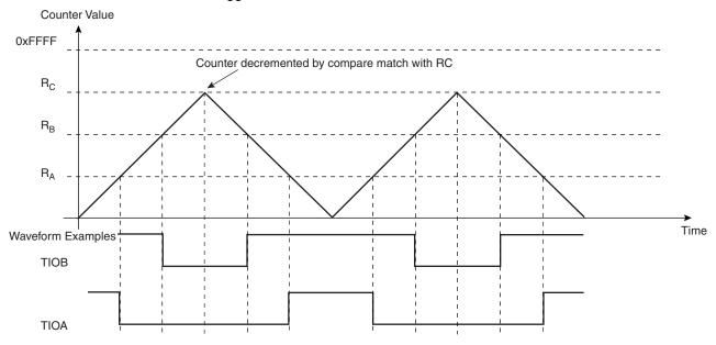
Figure 36-14. WAVSEL = 11 With Trigger
