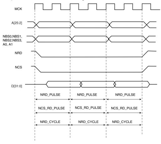
Figure 21-9. No Setup, No Hold On NRD and NCS Read Signals
