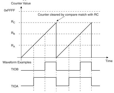
Figure 36-10. WAVSEL = 10 With Trigger
