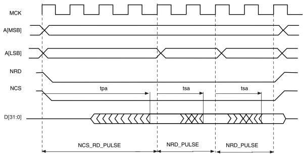
The NRD and NCS signals are held low during all read transfers, whatever the programmed values of the setup and hold timings in the User Interface may be. Moreover, the NRD and NCS timings are identical. The pulse length of the first access to the page is defined with the
