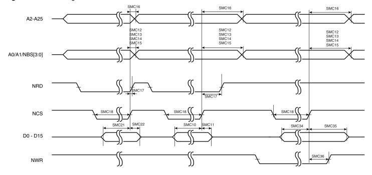
Figure 46-3. SMC Signals for NRD and NWR Controlled Accesses
