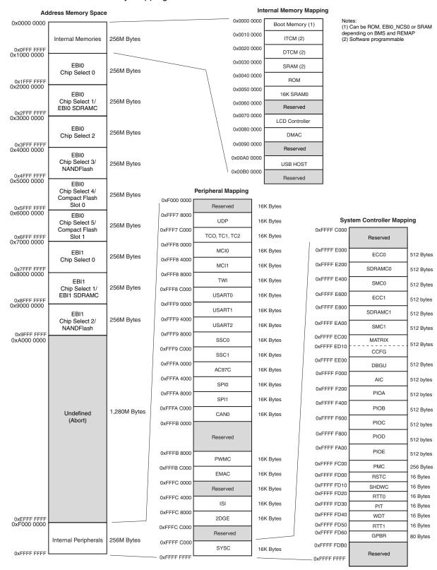
A first level of address decoding is performed by the Bus Matrix, i.e., the implementation of the Advanced High Performance Bus (AHB) for its master and slave interfaces with additional features.
