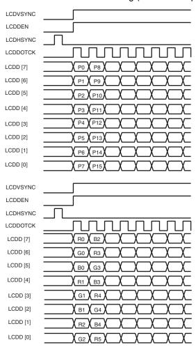
Figure 43-9. Dual Scan Monochrome and Color 8-bit Panel Timing (First Line Expanded View)
