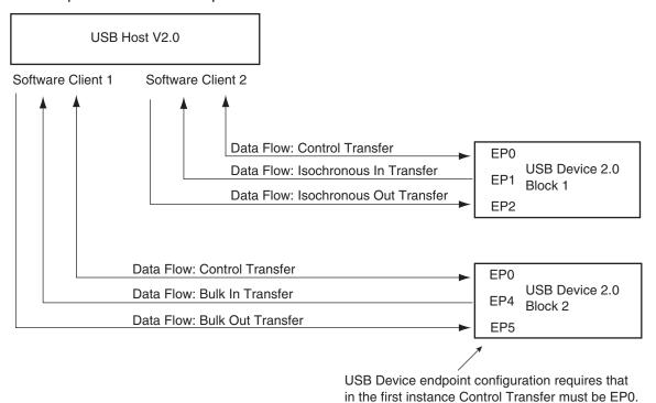
Figure 42-4. Example of USB V2.0 Full-speed Communication Control
