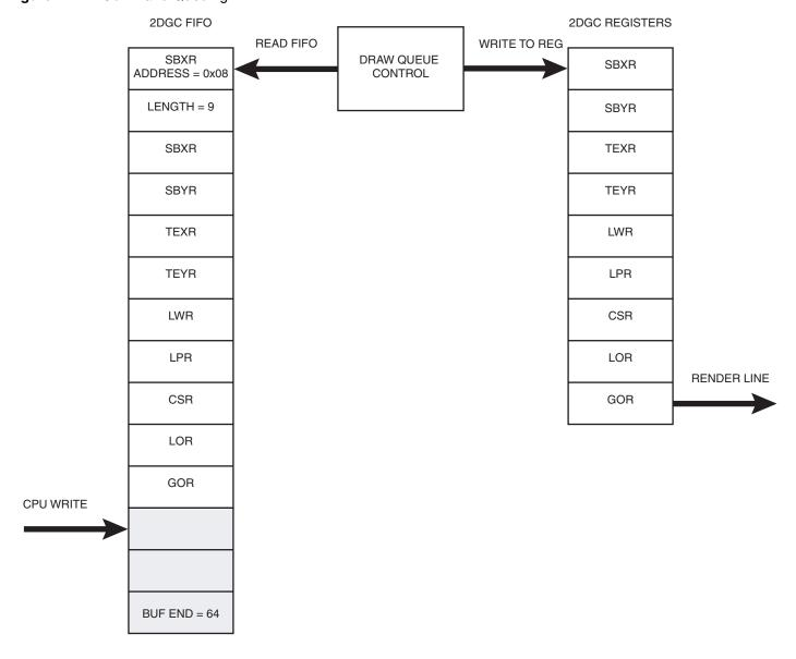
Recommended Procedure for Using the Command Queue
