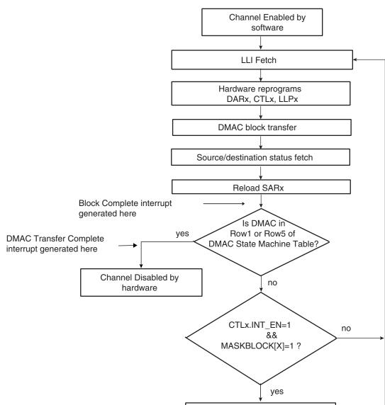
DMA Transfer Flow for Source Address Auto-reloaded and Linked List Destination Address
