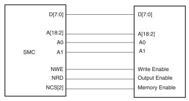
Figure 21-4. Memory Connection for a 16-bit Data Bus
