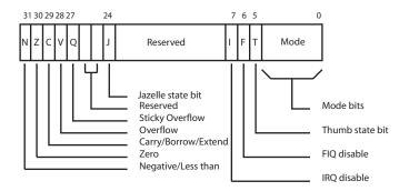
Figure 11-2 shows the status register format, where:
