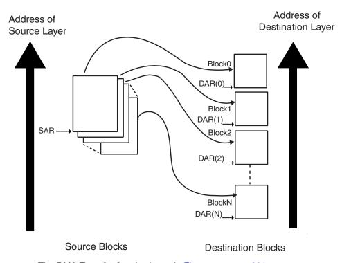
The DMA Transfer flow is shown in Figure on page 281
