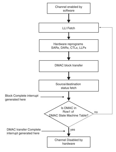
Multi-block Transfer with Source Address Auto-reloaded and Destination Address Auto-reloaded (Row 4)
