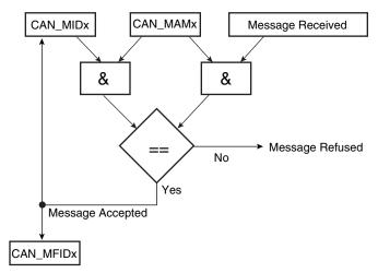
If a mailbox is dedicated to receiving several messages (a family of messages) with different IDs, the acceptance mask defined in the CAN\_MAMx register must mask the variable part of the ID family. Once a message is received, the application must decode the masked bits in the CAN\_MIDx. To speed up the decoding, masked bits are grouped in the family ID register (CAN\_MFIDx).
