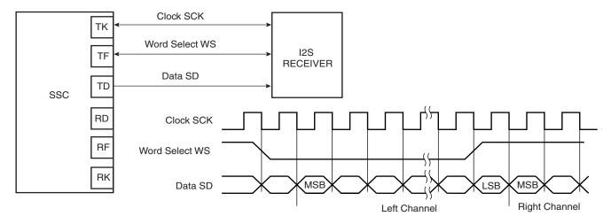
Figure 34-18. Codec Application Block Diagram
