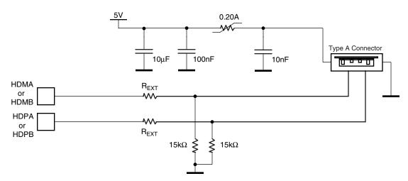
As device connection is automatically detected by the USB host port logic, a pull-down must be connected on DP and DM on the board. Otherwise the USB host permanently detects a device connection on this port.
