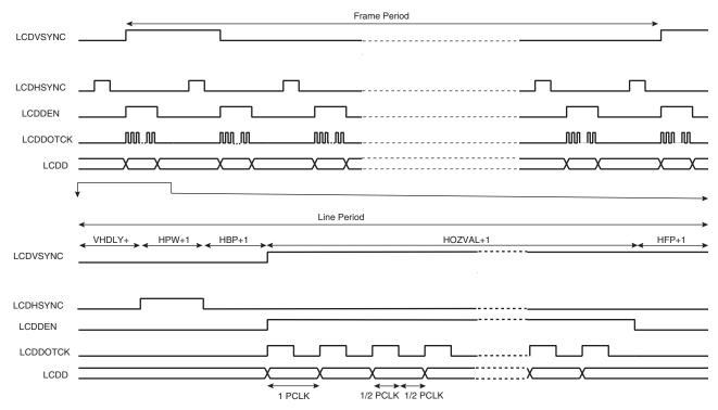
Figure 43-4. TFT Panel Timing, CLKMOD = 0, VPW = 2, VBP = 2, VFP = 1
