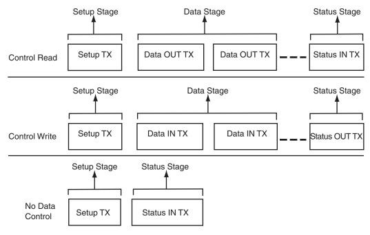
Notes: 1. During the Status IN stage, the host waits for a zero length packet (Data IN transaction with no data) from the device using DATA1 PID. Refer to Chapter 8 of the *Universal Serial Bus Specification, Rev. 2.0*, for more information on the protocol layer.
