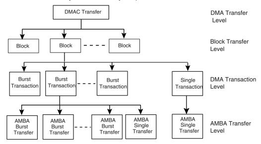
Figure 24-3. DMAC Transfer Hierarchy for Memory
