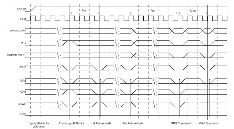
Figure 22-1. SDRAM Device Initialization Sequence
