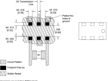
Dimensions are in Inches [Millimeters] Mounting Footprint
