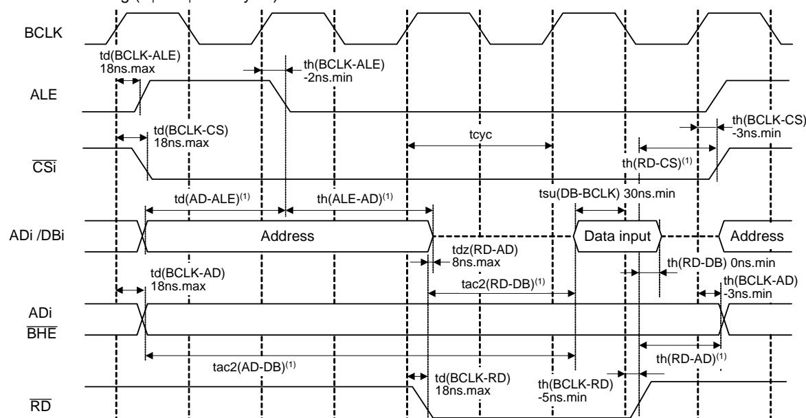
**Write Timing (2 $\phi$  + 2 $\phi$  Bus Cycle)**
