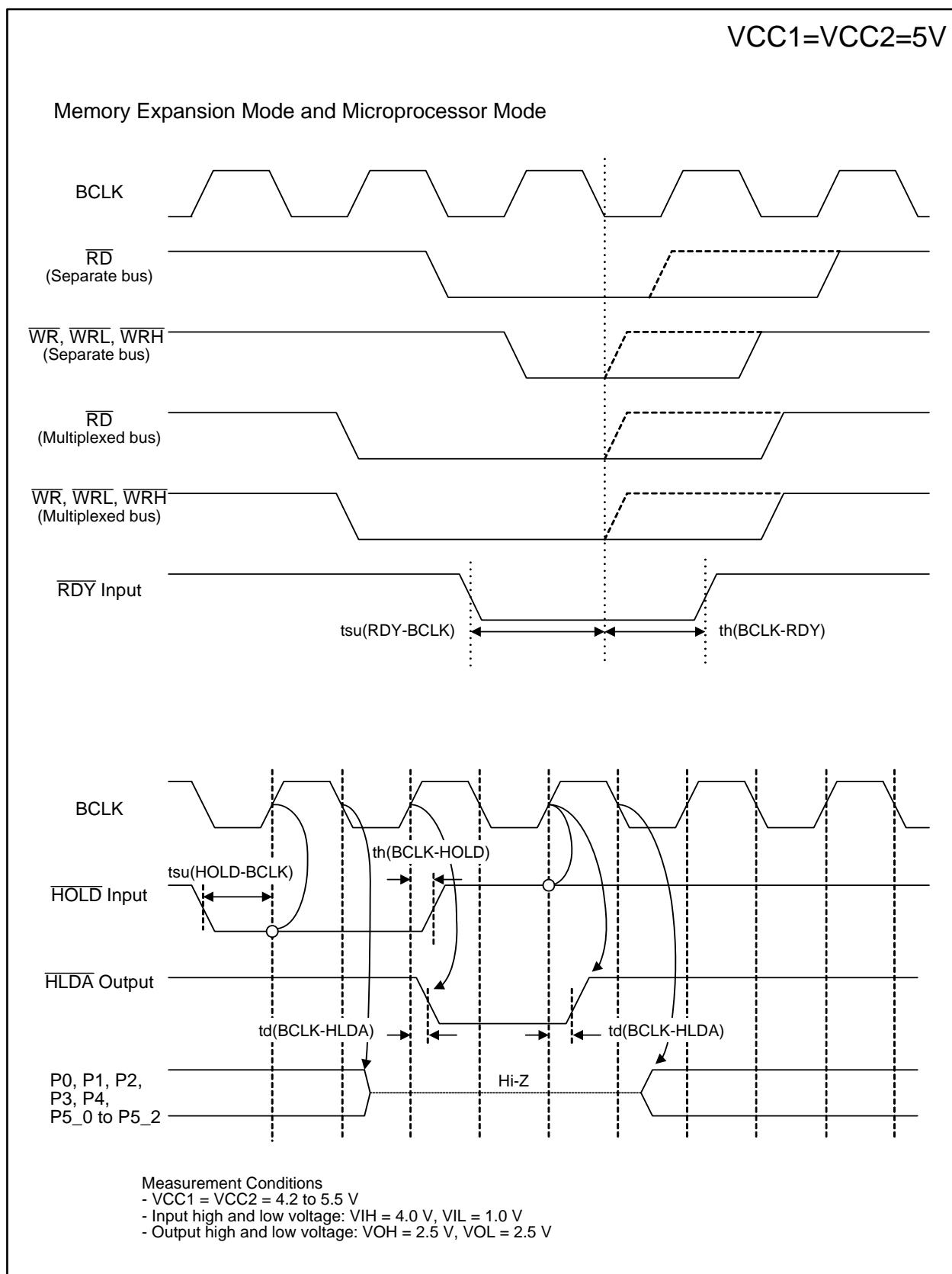
Figure 5.4 VCC1 = VCC2 = 5 V Timing Diagram (2/4)
