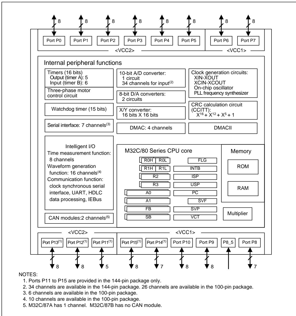
Figure 1.2 M32C/87 Group (M32C/87, M32C/87A, M32C/87B) Block Diagram
