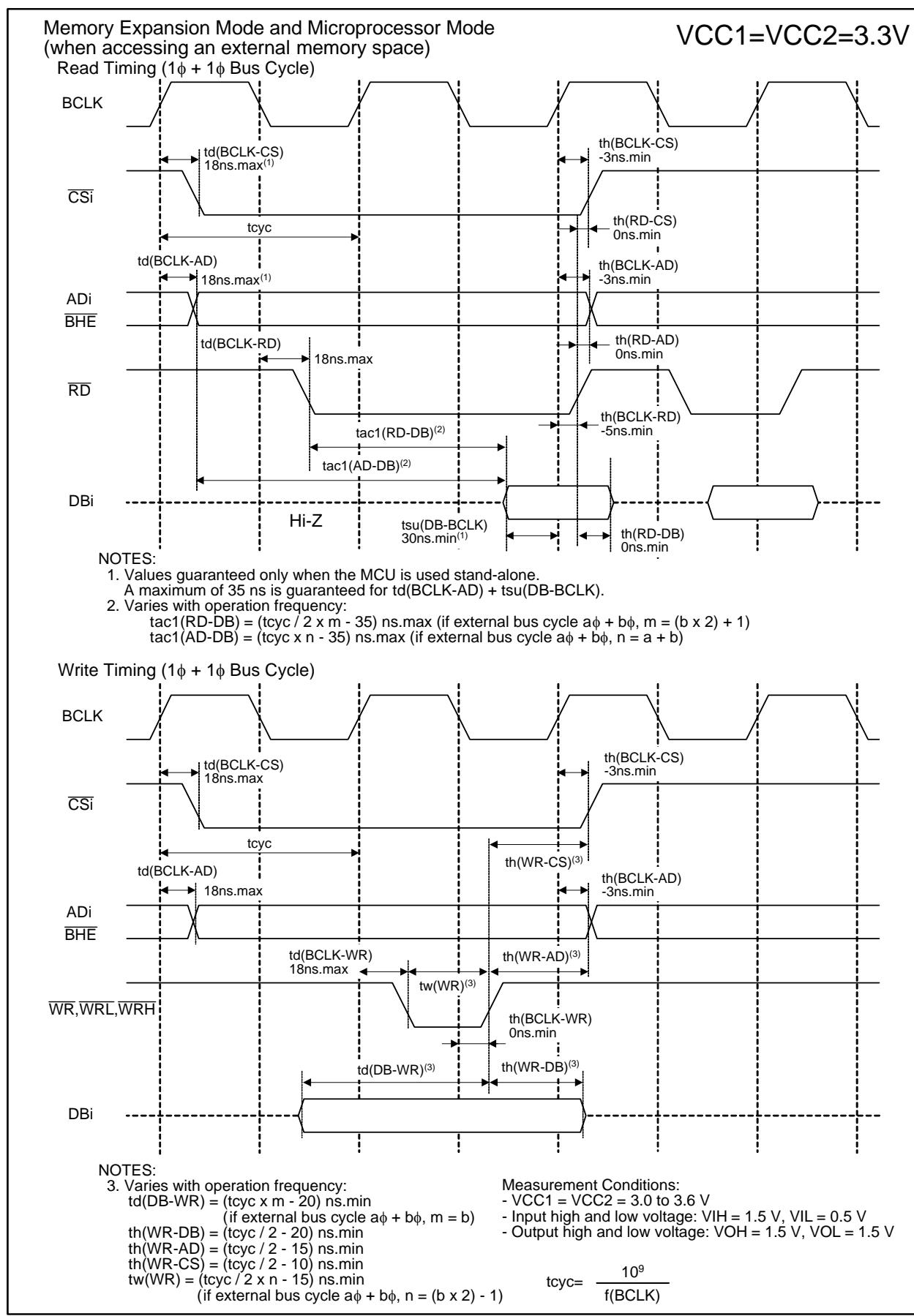
**Figure 5.9 VCC1 = VCC2 = 3.3 V Timing Diagram (3/4)**
