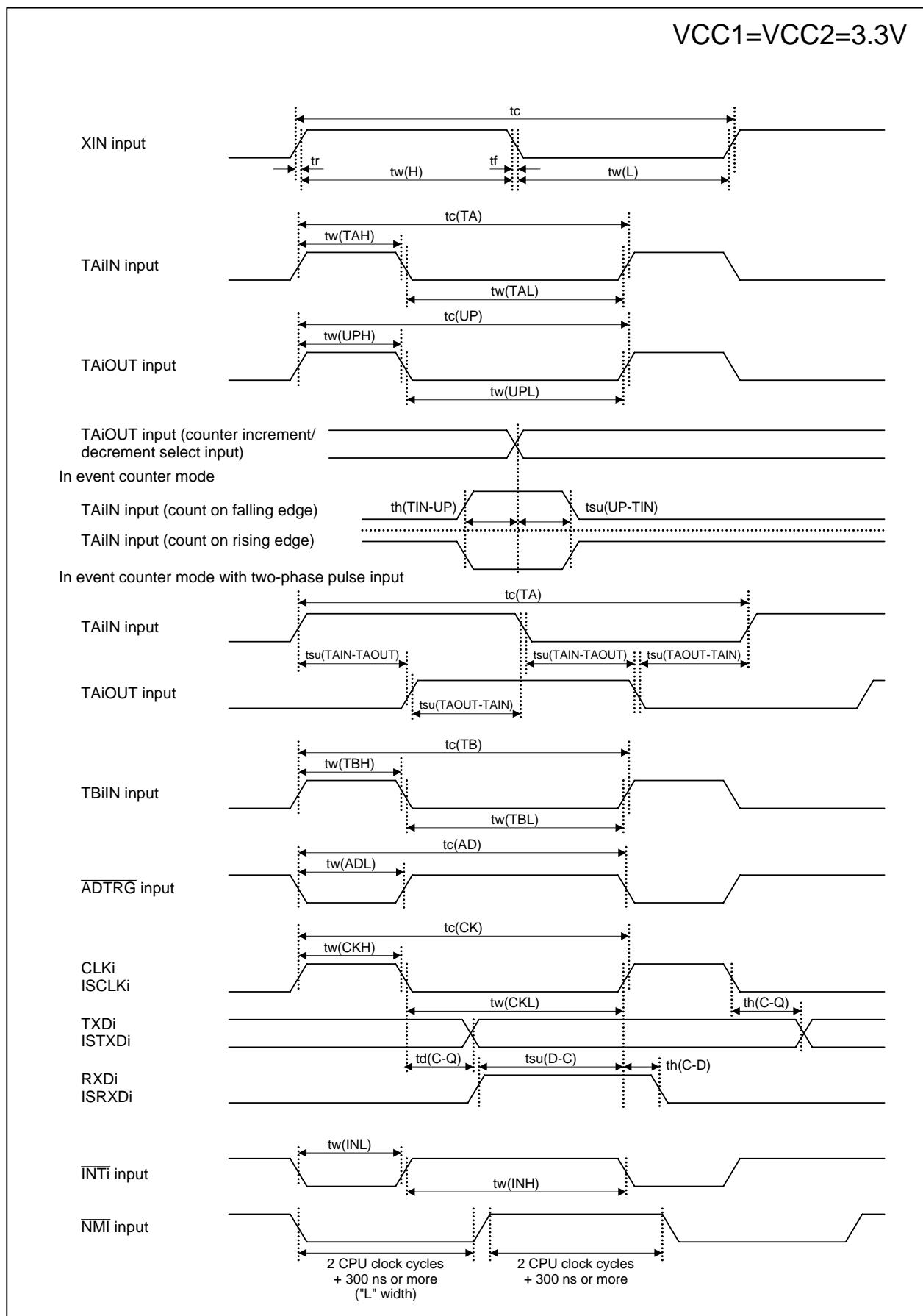
**Figure 5.7      VCC1 = VCC2 = 3.3 V Timing Diagram (1/4)**
