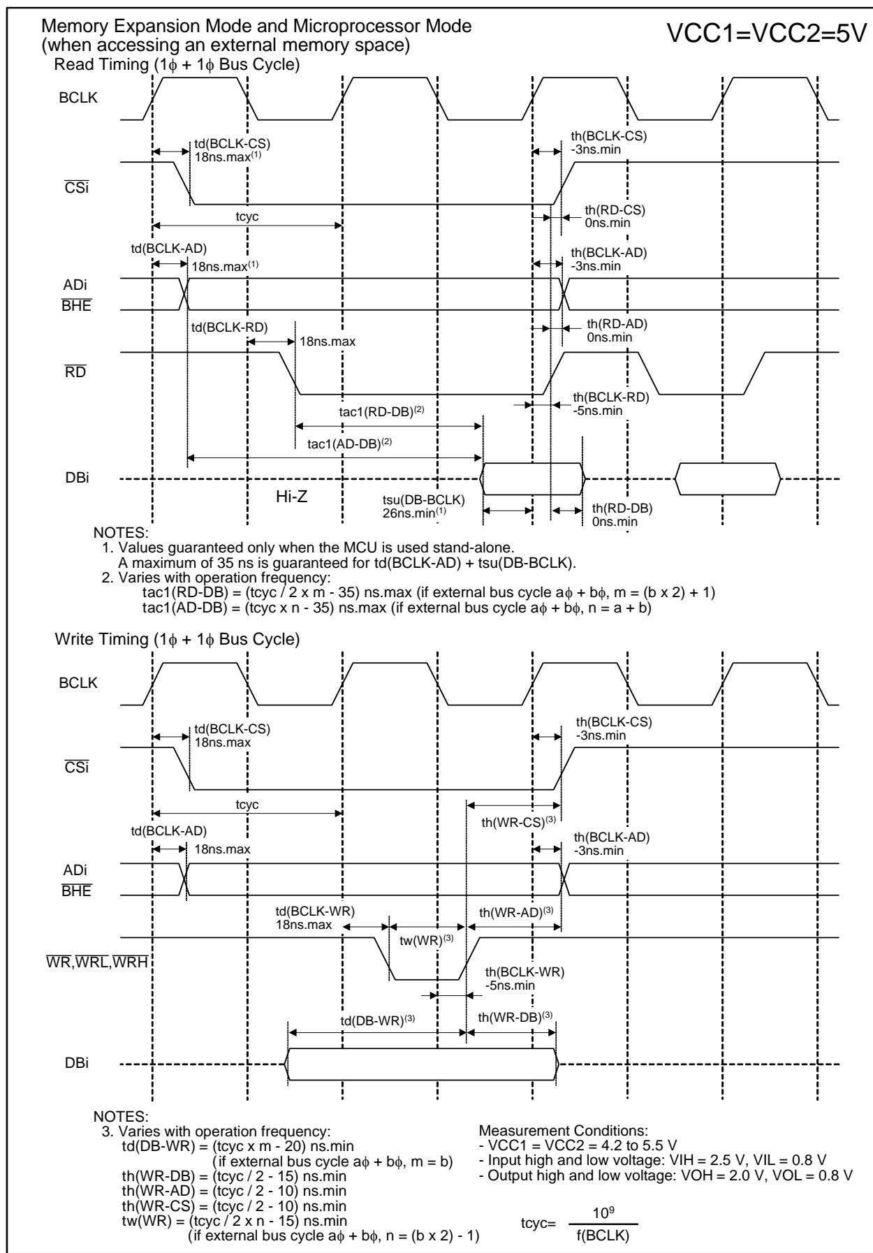
**Figure 5.5 VCC1 = VCC2 = 5 V Timing Diagram (3/4)**
