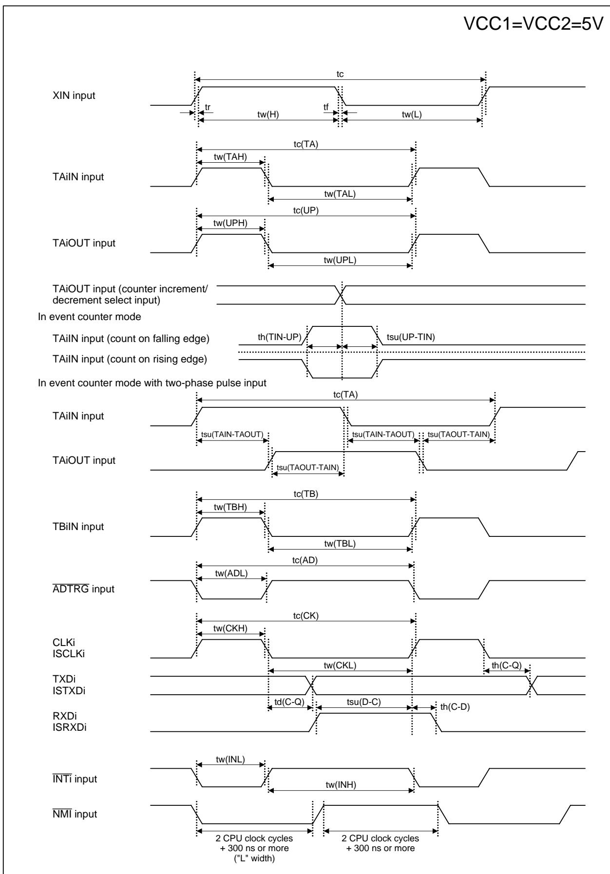
**Figure 5.3      VCC1 = VCC2 = 5 V Timing Diagram (1/4)**
