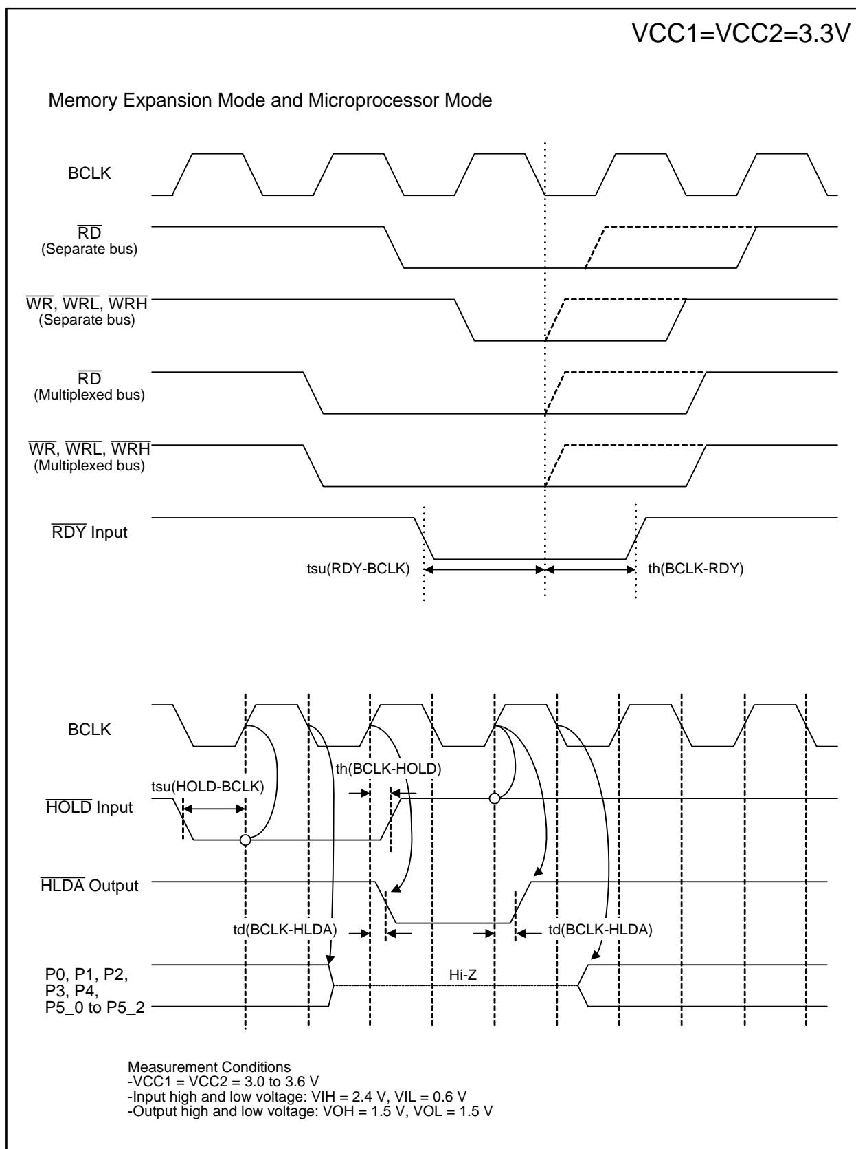
Figure 5.8 VCC1 = VCC2 = 3.3 V Timing Diagram (2/4)
