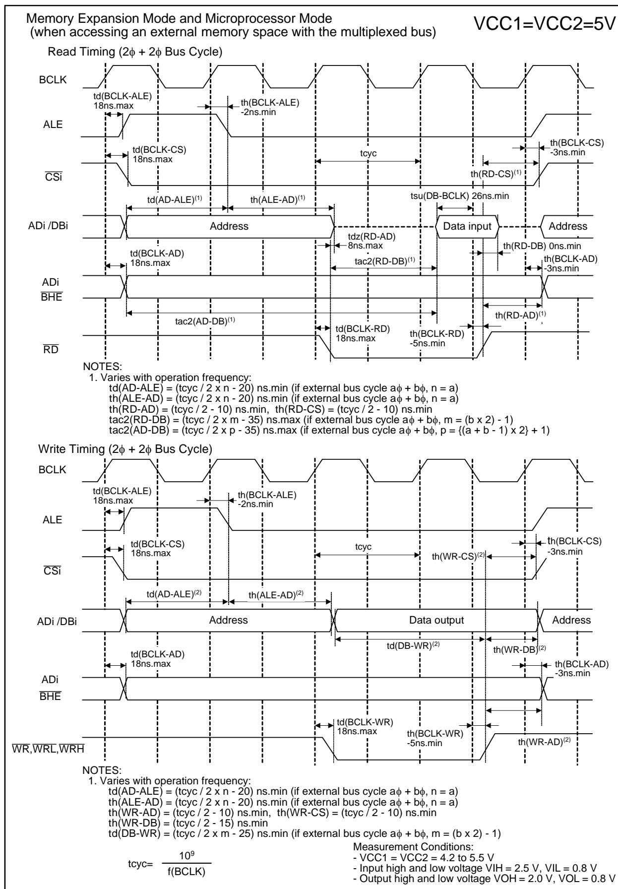
**Figure 5.6 VCC1 = VCC2 = 5 V Timing Diagram (4/4)**
