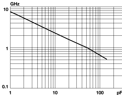
Typical Self Resonant Frequency vs. Capacitance Accu-F®/Accu-P® 0805
