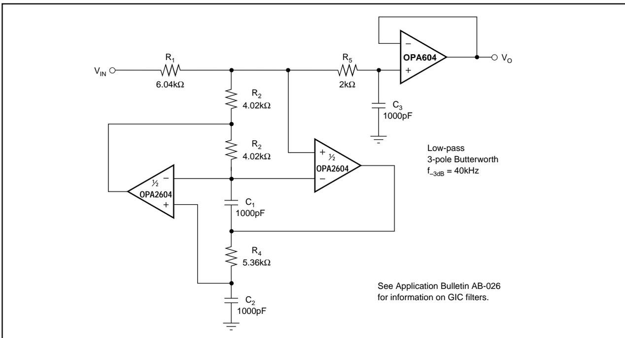
FIGURE 5. Three-Pole Generalized Immittance Converter (GIC) Low-Pass Filter.
