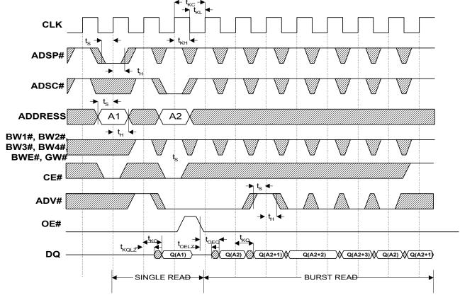
Note: 27.  $\overline{CE}$  active in this timing diagram means that all chip enables  $\overline{CE}$ , CE2, and  $\overline{CE2}$  are active.
