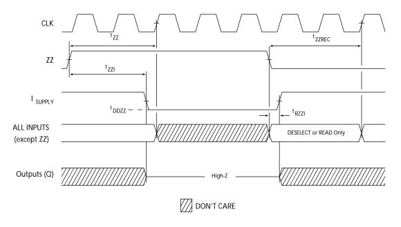
25. Device must be deselected when entering ZZ mode. See truth table for all possible signal conditions to deselect the device. 26. DQs are in high-Z when exiting ZZ sleep mode.
