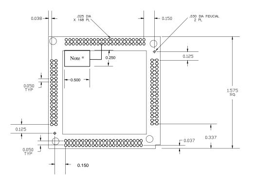
\* Note: Ground shield to isolate RTC XTAL from EMI
