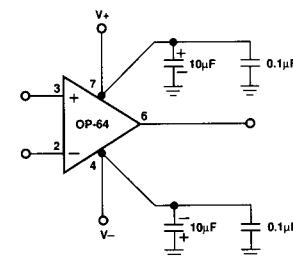
**FIGURE 1:** Proper power supply bypassing is required to obtain optimum performance with the OP-64.
