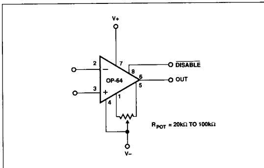
FIGURE 2: *Input Offset Voltage Nulling***OFFSET VOLTAGE ADJUSTMENT**
