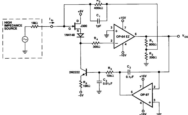
FIGURE 9: Fast Transimpedance Amplifier
