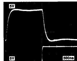
FIGURE 10: Output of the Fast Transimpedance Amplifier
