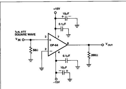
**FIGURE 7:** Overdrive Recovery Test Circuit
