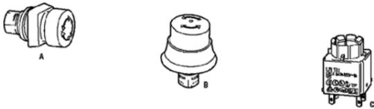
**Contact Rating:** Silver — 6 amps at 250 VAC; Gold — 250 mA at 42 VAC/VDC. **Contact Resistance:** Silver — 20 milliohms; Gold — <50 milliohms. **Operating Temperature:** -25°C to 70°C. **Operating Life:** 30,000 cycles. **Terminals:** Quick connect 2.0 x 0.8 tin plated. **Degree of Protection:** IP65, dustproof, water splash, dew condensation.
