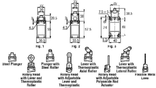
Body, head and actuator arm are pre-assembled with only one part number to order. Standard limit switches have a SPDT-DB positive opening contacts. Manual reset limits have a slow break SPDT-DB with positive opening contacts. All models feature a 1/2" NPT fitting. Metric fittings are available by request.
