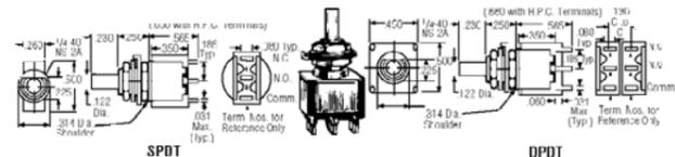
Specifications. Contact Rating: 5 A resistive (1 pole), 1 A resistive (2 pole) @ 125 VAC or 28 VDC (UL listed) or 0.4 Volt-amp (VA) maximum @ 28 V max. (AC or DC), 60,000 cycles minimum at full load resistive. Center and End Contact: 1 and 5 A, brass, silver inlay and gold flash for solderability. .4 VA — brass, 50 millionth gold plated over nickel. Epoxy seal is standard. Caps sold separately.
