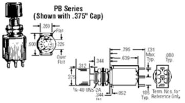
**PB Series Pushbutton Switches**
