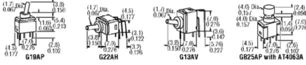
Micro-subminiature, PCB mountable, antistatic, washable, patented Sliding Twin Crossbar (STC) contact mechanism, plus molded-in, epoxy sealed terminals with 0.100" x 0.100" spacing. **Electrical Capacity:** 0.4 VA maximum @ 28 V AC/DC maximum. **Electrical Life:** 100,000 operations minimum for on-none-on and on-off-on toggles; 50,000 operations minimum for other toggle circuits as well as for pushbutton circuits.
