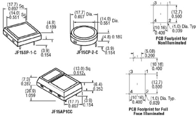
Extremely low profile and completely sealed dome contact. SPST contacts with strapped terminals allow X-Y coding on 1-sided PCB. Off-Momentary on circuit. **Resistive Load:** 50 mA @ 24 V DC. **Electrical Life:** 500,000 operations min. **Total Travel:** 0.031" with sculptured actuator, 0.16" with flush actuator. **Operating Force:** 200 grams with sculptured actuator, 350 grams with flush actuator. **Contact Bounce:** 0.1 millisecond max.
