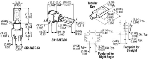
Single pole. Straight PC with bracket. Gold contacts. Two polyacetal keys supplied with each switch. **Electrical Capacity:** 0.4 A @ 28 VAC/DC. **Dielectric Strength:** 500 VAC minimum. **Mechanical Life:** 30,000 cycles minimum. **Electrical Life:** 20,000 cycles minimum. **Operating Torque:** 2.039 grams-cm. **Ambient Temperature:** -25°C through +70°C. **Angle of Throw:** 90° for 3 position models and 45° for 5 position models.
