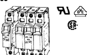
Trip free multi-pole thermal-magnetic circuit breaker rated 480 VAC 65 VDC. DIN rail mounting (35 mm). Add-on modules include — auxiliary and signal contact options; remote trip release option. Other rated currents and 4-pole option available.
