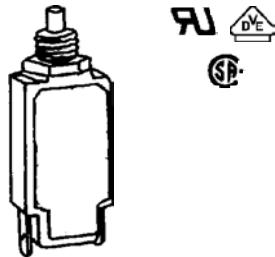
Trip-free single pole push to reset. Rated 240 VAC, 48 VDC. 6.3 x 0.8 mm quick connect terminals. Options include shunt terminal up to 6 A; silver contacts meet UL 1077 up to 12 A ratings; and trip band indicator. Dust cover also available.
