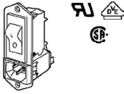
Series PEM 45 power entry module combines an AC inlet, circuit breaker for equipment, and optional RFI filter. The circuit breaker provides manual reset of the circuit, 1 or 2-pole thermal overload protection, or no-bi-metal for on/off switching only (white switch I/O embossed lettering). Optional undervoltage release. Approved by UL, CSA up to 15 amps at 125 and 250 volt, and VDE up to 10 amps 250 volt.
