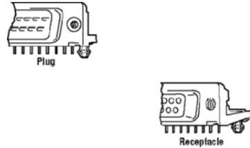
590 mount with boardlock. **Front Shell:** Steel, tin plated. **Housing:** Black thermoplastic, 94V-0 rated. **Threaded Inserts:** Zinc. **Contacts-Pin:** Brass. **Sockets:** Phosphor bronze plated with 0.000030 (0.00076) min. gold on mating end, tin-lead on termination end, all nickel underplated.
