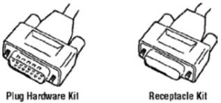
**Material and Finish:** Connector shell — steel, tin plated; Connector insert — thermoplastic, 94V-0 rated, black; Shields — steel, tin plated. **Kits include:** Connector, inner shield, outer shield, enclosure and two jackscrews. Contacts and ferrules must be ordered separately.
