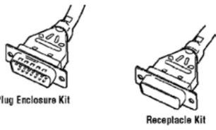
**Material and Finish:** Connector shell — steel, tin plated; Connector insert — thermoplastic, 94V-0 rated, black; Shields — steel, tin plated. **Kits include:** Connector, inner shield, and outer shield. Contacts and ferrules must be ordered separately.
