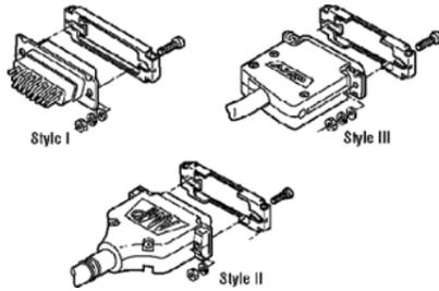
**Material and Finish:** Slide latches — stainless steel; 4-40 screws, washers and hex nuts — steel, zinc-plated yellow chromate; 2-56 screws, washers and hex nuts — steel, zinc-plated clear chromate.
