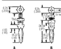
**Material:** Banana plug body — Brass; Spring — One piece heat treated beryllium copper. Fits standard 4.22 mm (0.166) dia. banana jack. **Finish:** Nickel plated. **Rating:** 5000 WVDC, 15 amps.
