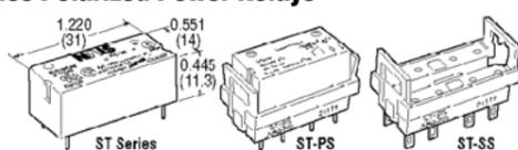
Sealed for automatic wave soldering and cleaning. **Initial Contact Resistance:** 30 milliohms. **Row Spacing:** 0.400" (10.16 mm). Gold-plated silver alloy contacts. **Rated:** 8 A, 200 VA. **Switching Power:** 150 W. **Switching Voltage:** 380 VAC. **Nominal Operating Power:** 240 mW. **Shock Resistance:** 20 G. **Ambient Temperature:** -40°C to +60°C. UL/CSA.
