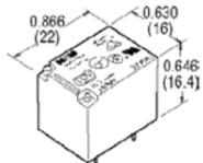
10 A universal terminal footprint. **Nominal Operating Power:** 360 mW. **Pick Up Voltage:** 70% nominal voltage, sealed. **Maximum Switching Power:** 1250 VA. **Ambient Temperature:** -40°C to +70°C. UL recognized, CSA certified, TÜV approved.
