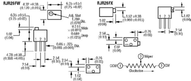
Listed on DESC QPL per high-rel Mil-R-39035. Thin body profile, multi-turn, cermet trimmer with infinite resolution. Outstanding humidity resistance and low contact resistance. Sealed to withstand wave soldering and board washing processes. **Resistance Tolerance:** ±10%. **Power Rating:** 0.25 watt at 85°C. **Adjustment Tool:** H-90.
