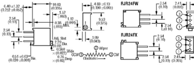
Listed on DESC QPL per high-rel Mil-R-39035. Thin body profile, multi-turn, cermet trimmer with infinite resolution. Wiper riding mechanism clicks at the end of rotation. Built-in standoffs. Sealed to withstand wave soldering and board washing processes. **Resistance Tolerance:** ±10%. **Power Rating:** 0.5 watt at 70°C. **Adjustment Tool:** H-90.
