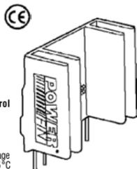
Crydom's PowerFin™ series delivers the highest ratings of any single in-line package (SIP). The integral heat sink design can operate at 25 amps RMS in forced air at 85°C case temp. With natural convection in free air, it rates 10 amps RMS at 25°C ambient. Operating Temperature Range: -30°C to 80°C. Isolation Voltage (Vrms): 2500.
