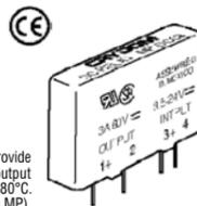
Available in 3 Arms and 4 Arms ratings, all are SPST-NO PC-mount relays that provide greater packaging density and compatibility with pin out of Series 6 and OAC output modules. Internal snubber included. Operating Temperature Range: -30°C to 80°C. Isolation Voltage (Vrms): 4000. PX models available in the MP package (see Series MP). Dimensions (L x W x H): 1.7 x 0.4 x 1.0 (43.1 x 10.2 x 25.4 mm).
