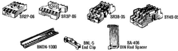
Snap-mount sockets are designed to mount on BNDN-1000 mounting rail. The built-in mounting clip eliminates mounting hardware and reduces mounting time by eighty percent. For spacing between adjoining sockets, use SA-406 DIN rail spacer. **Spacers:** 0.197" in width. Spacing can be adjusted according to the amount of spacers added. To prevent sideward movement, use BNL-5 end clip at each end of socket row.
