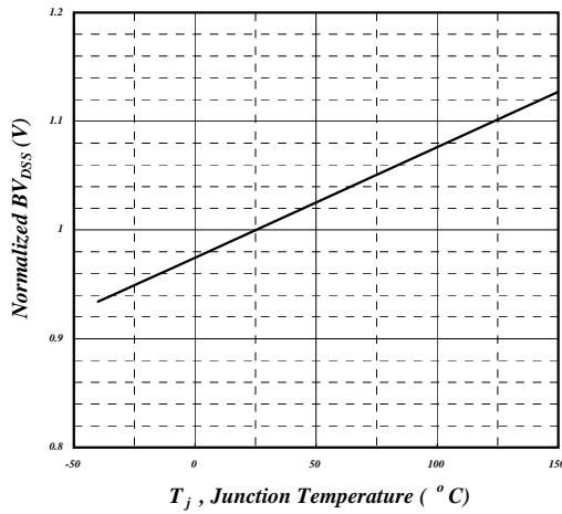
Fig 3. Normalized  $BV_{DSS}$  v.s. Junction Temperature
