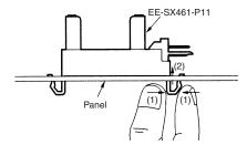
Pressed mounting holes are ideal for mounting the Photomicrosensor. When mounting the Photomicrosensor to a panel that has pressed mounting holes for the Photomicrosensor, be sure to mount the Photomicrosensor on the pressing side of the panel, otherwise it may be difficult to mount the Photomicrosensor and an insertion force of five to six kilograms may be required.
