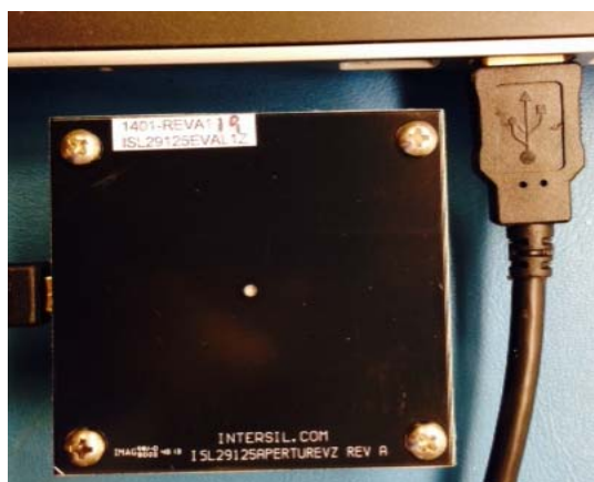
FIGURE 7. ISL29125 EVAL BOARD CONNECT TO PC BY MINI USB
