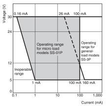
However, even when using microload models within the operating range shown above, if inrush current or inductive voltage spikes occur when the contact is opened or closed, it may increase contact wear and so decrease the service life. Therefore, insert a contact protection circuit where necessary.
