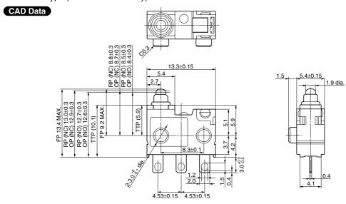
Angle terminal type (3 mm standard type only) mm General tolerance: ±0.25
