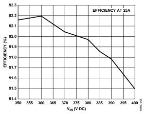
Figure 66. Efficiency vs. V<sub>IN</sub>
