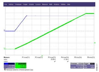
Figure 18. Startup at 385 V DC, 25 A Load (1 A/µs Slew Rate) Green Trace: Output Voltage, 2 V/div, 10 ms/div Blue Trace: Load Current, 10 A/div, 10 ms/div
