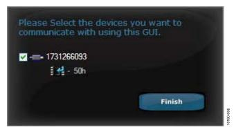
Figure 7. ADP1046 Address of 0x50 in the GUI
