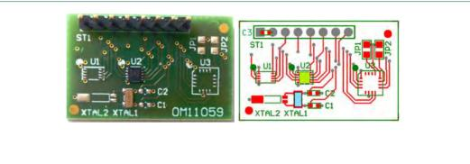
Fig 3. Picture and layout of demo bard OM11059
