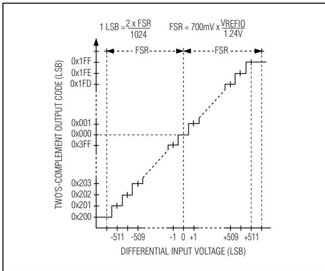
Figure 6. Two's-Complement Transfer Function ( $\bar{T}/B = 0$ )
