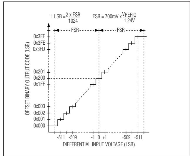
Figure 7. Binary Transfer Function ( $\bar{T}/B = 1$ )
