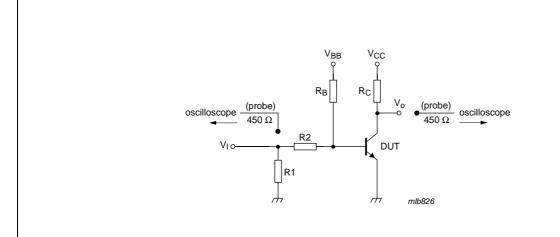
$$\begin{split} V_i = 9.5 \ V; \ T = 500 \ \mu s; \ t_p = 10 \ \mu s; \ t_r = t_f \leq 3 \ ns. \\ R1 = 68 \ \Omega; \ R2 = 325 \ \Omega; \ R_B = 325 \ \Omega; \ R_C = 160 \ \Omega. \end{split}$$
